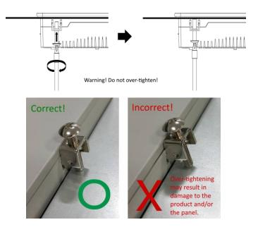
4. Repeat for each bracket and verify that the display is properly mounted and secured to the panel.
