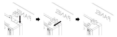
3. Tighten the bracket mounting bolts to secure the display to the panel. The recommended torque is 0.4
