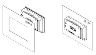
2. Insert the panel mount brackets into the bracket mounting holes as shown in the image below, pulling the bracket to lock it into place.
